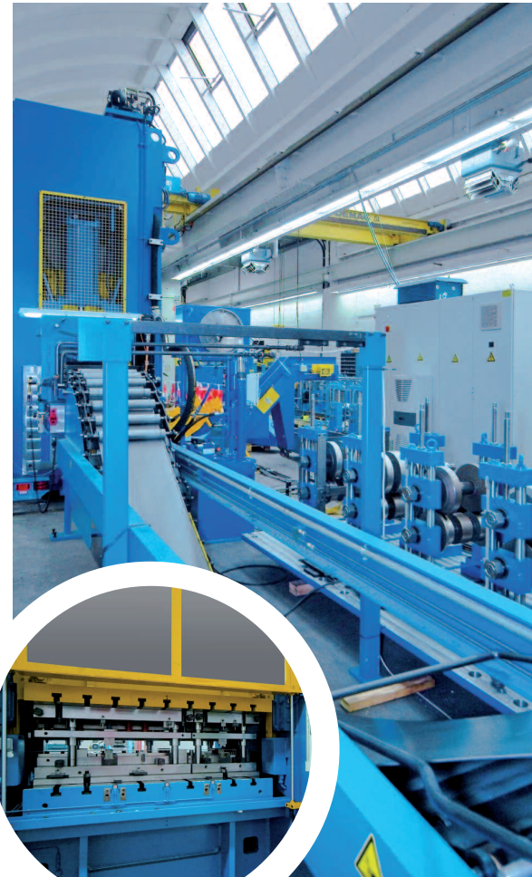
Pre-punch system with integrated mechanical press
